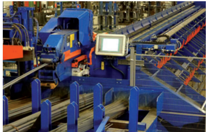
Combiline measuring and in-feed device for precise cut lengths combined with the Autender counter and insertion system, plus pallet system
