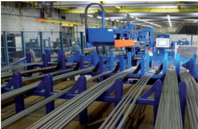
No employees are needed for operating the concrete reinforcing steel cutting system from Pedax
