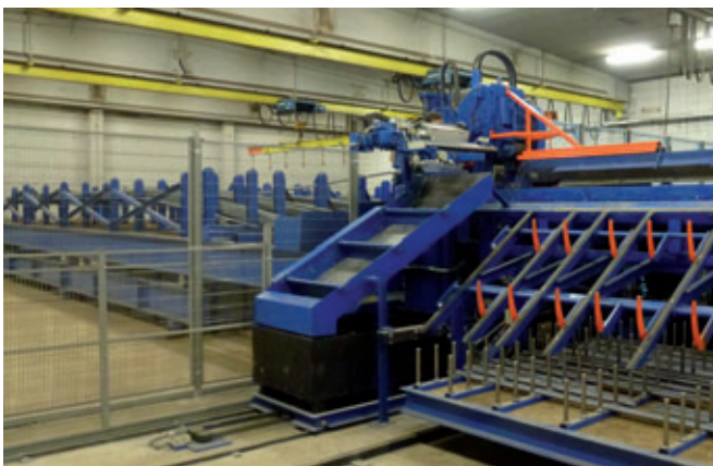
View of the pallet storage unit and the automatic collector for short cut lengths
