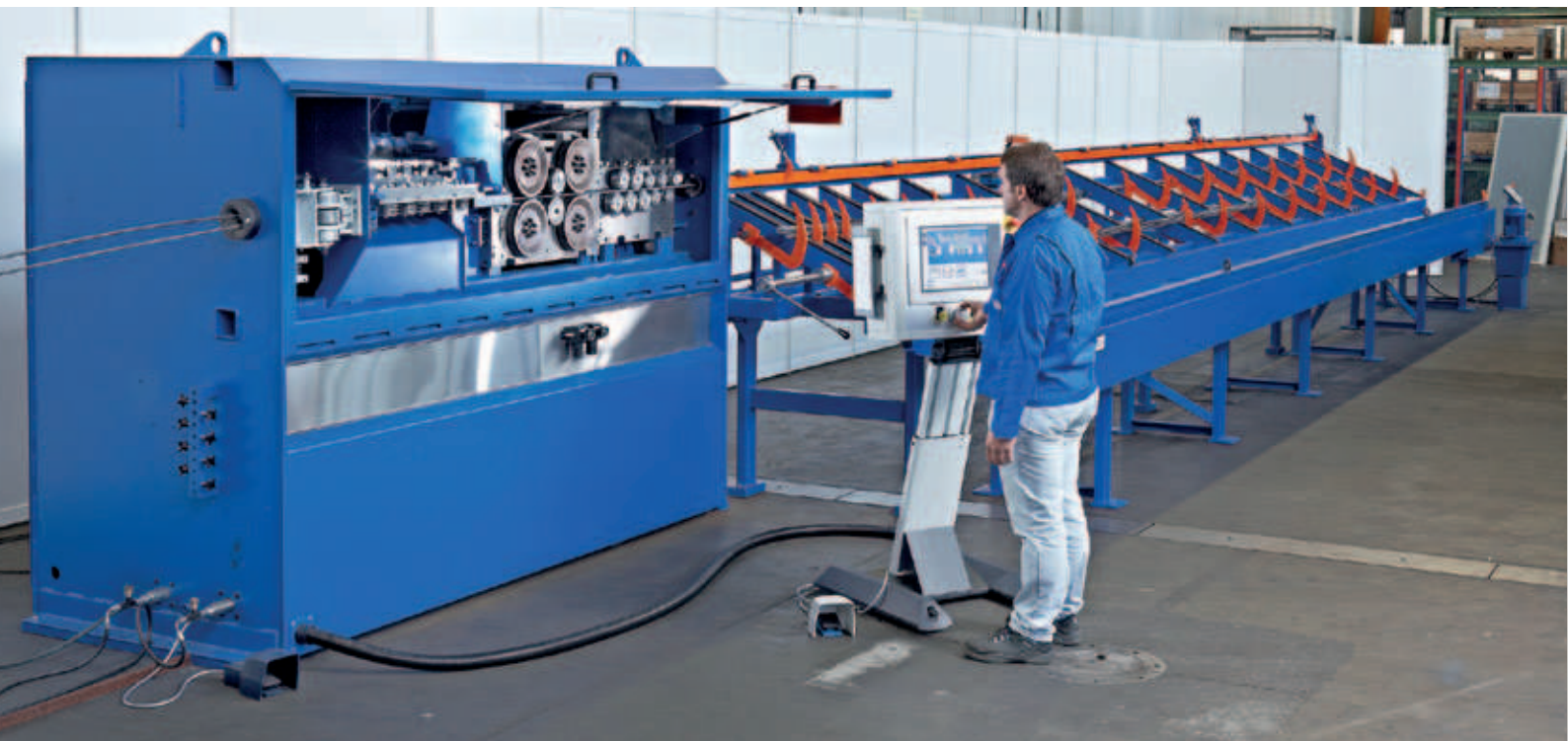
Twincut 12 roller straightening machine equipped with a rebar storage unit for lengths that have already been straightened and cut
