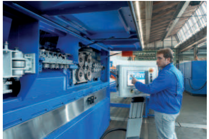
An additional feed unit facilitates inserting the wires into both roller straightening units, which are set up both vertically and horizontally. These roller straightening units have been well tried and tested in Pedax stirrup bending machines
