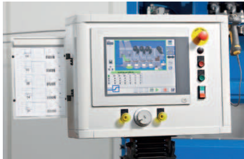
A logically structured user interface with a B & R touchscreen and, as an option, a laser scanner for transferring data directly from the label
