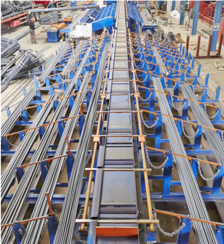
Figure 3: View of the positioning track and the collection boxes for fixed lengths located on both sides. The collection boxes each offer 6 compartments and thus sufficient storage space for different batches.
