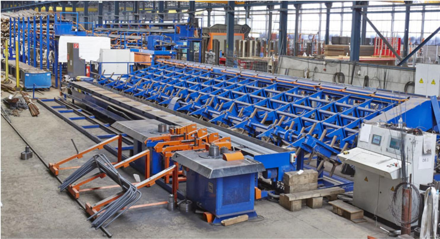
Figure 2: Bending lengths are transported to double bending machines via pocket systems and transverse chain conveyors. This system includes two double benders.
