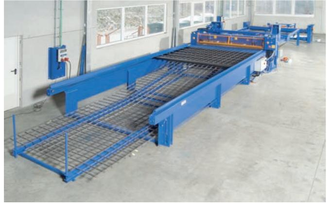
*Mafix mesh cutting system with feed and removal system*
