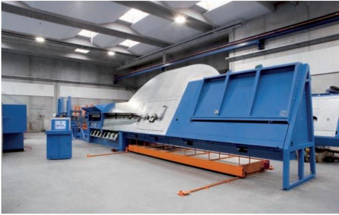
*Twinmaster 20 reinforcing steel processing centre - equipped with anti-stress unit and anti-twist device, and new straightening mechanism with separate drives. Processes coil material up to 20 mm diameter.*
